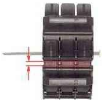
... and afterwards. The red lines indicate by just how much the segment have been tightened
